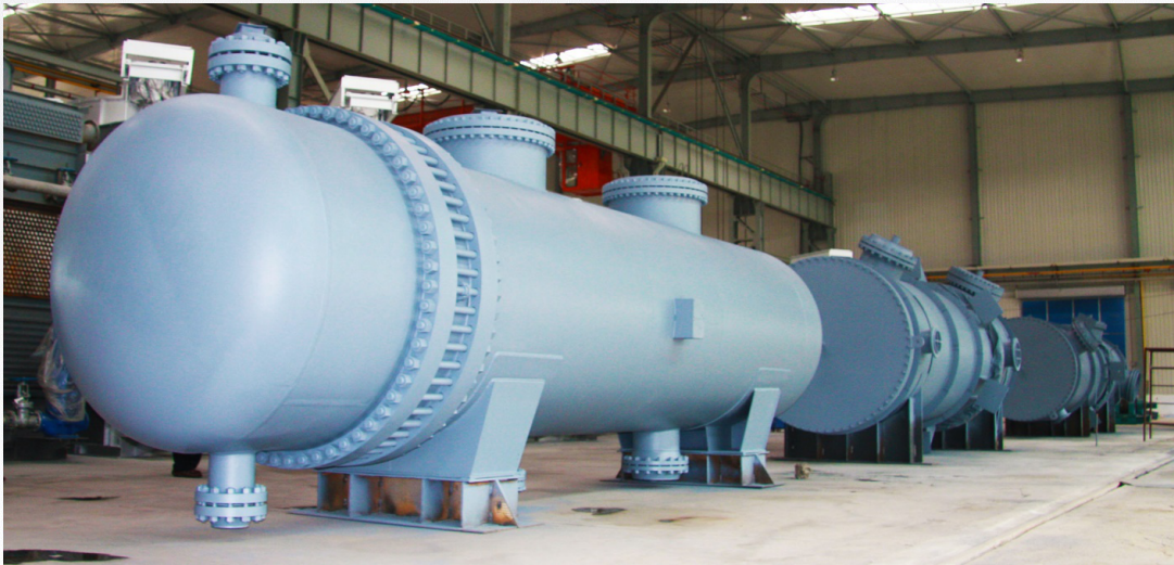
Left: A high efficiency heat exchanger with UOP high flux tube
