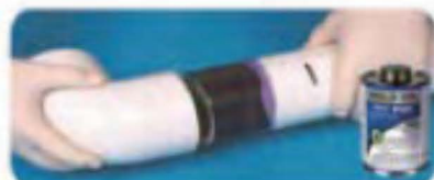
11. While inserting, twist 1/8 to 1/4 turn until reaching socket bottom, Hold for 30 seconds to eliminate movement 边推边旋转 1/4 圈至底部, 按住 30 秒 防止反弹
